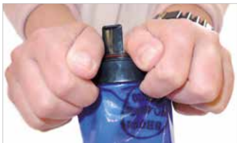
5.5 Press the glove and Oval Spanner Ring so that it bottoms in the Oval Glove Ring. Perform this procedure 360° around the ring.
