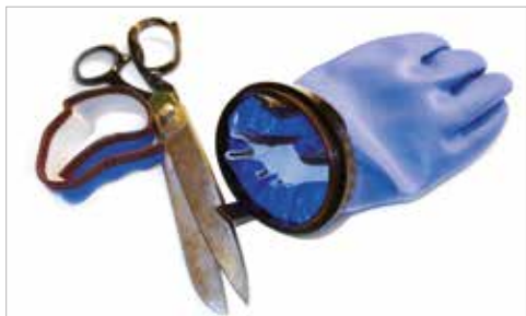
5.7 For the best comfort and performance, cut back excess glove material. Our recommendation is to remove enough excess material to prevent interference with the latch arms.
