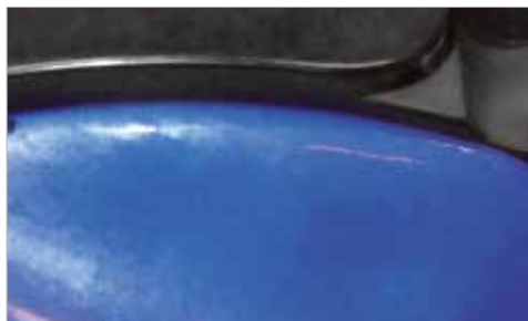
5.4 Check for creases on the glove continuously when pressing the Glove/Oval Spanner Ring into final position. The glove should be positioned as displayed in this image.
